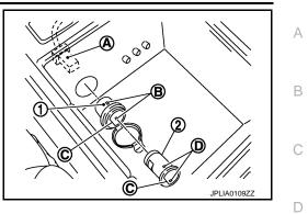
INSTALLATION Install in the reverse order of removal. **NOTE:** Align the cut outs of inner socket and ring.
